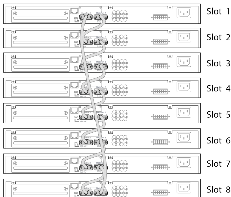
Figure 39: SummitStack Cable Connections Using Eight Switches with Integrated SummitStack Ports
